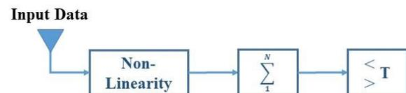
**Figure 2: Block diagram for optimal likelihood ratio binary hypothesis test**
